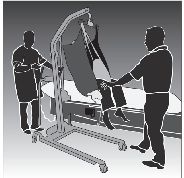
Figure 44 – A mobile hoist reduces the forces required to transfer a patient
