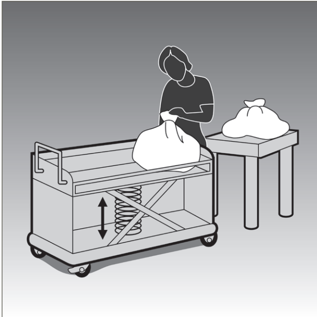
Figure 46 – A self-adjusting base in the laundry tub reduces the need for bending and twisting during unloading
