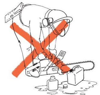
Figure 48: Do not start saw near fuel supply
