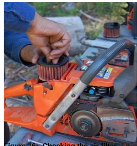
Figure 16: Checking the air filter
