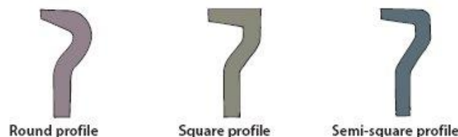
Figure 34: Different cutter profiles
