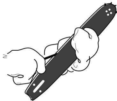
Figure 29: Cleaning the groove
