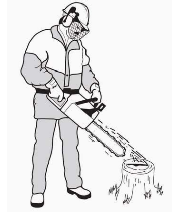
Figure 51: Checking for chain lubrication
