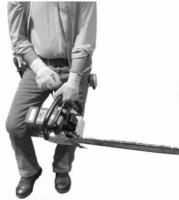
Figure 50: Leg lock method
