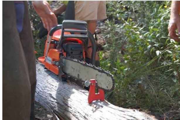
Figure 38: Using a stump vice
