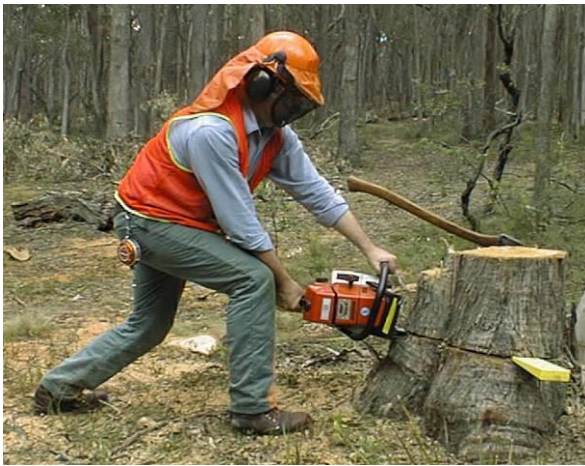
Figure 61: Horizontal cutting technique
