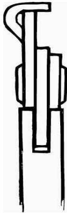
Bar gauge helps support chain
