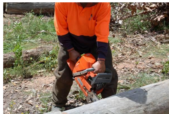
Figure 58: Keep a balanced stance and firm grip
