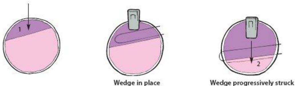
Figure 72: Bridging cut using a wedge
